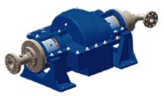
Pitot tube, between bearings **Capacity:** 450 gpm / 102 m³/h **Head:** 4,920 ft / 1,500 m **Pressure:** 2,175 psig / 150 bar **Temp Range:** 250° F (120° C)
