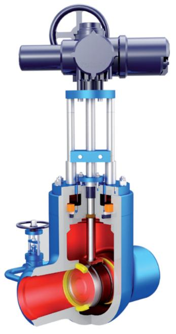
The Hopkinsons Venturi design is used when a slightly higher pressure drop is acceptable. The well-established principle of fluid flow through a Venturi is used in order to minimise pressure drop. Venturi valves incorporate the design feature of an eye follower. In the fully open position the eye follower bridges the gap between the seats thus giving a smooth flow path and completing the Venturi profile.
